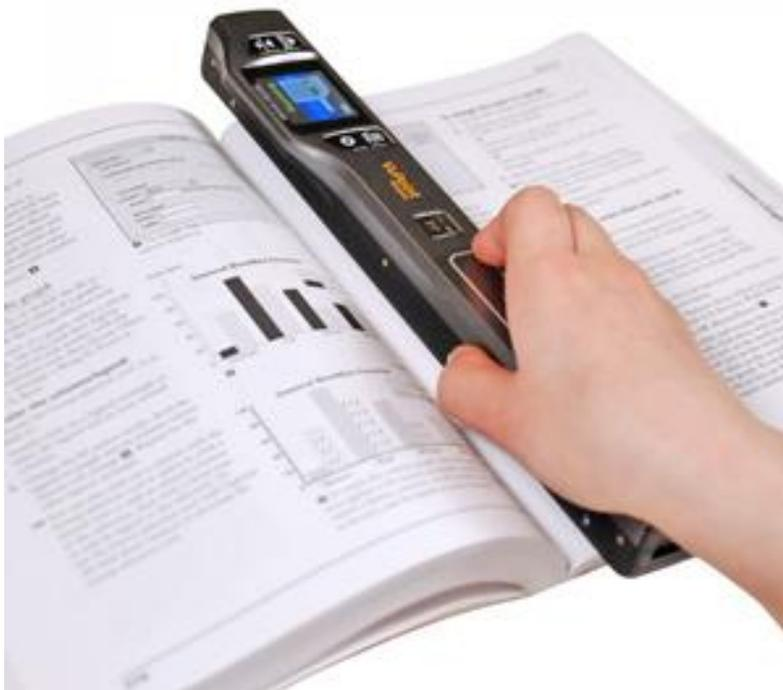
The scanning process is pretty straight forward, just turn the Magic Wand on with the on/off button for a few seconds until it turns on; then press the on/off button again to start a scan, do the scan, then turn the on/off button again to stop the scan. The LED keeps you informed or the number of scans
