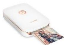
Let's start with the **HP Sprocket** which will create 2x3-inch prints from your favorite social media sites. This little printer uses pulses of heat to activate layers of crystallized dyes in Zink paper. You can print from Bluetooth and NFC wirelessly or you
