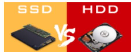
The type of storage your computer uses matters for several reasons. Hard disk drives (HDD) and solidstate drives (SSDs) are the two main storage options to consider. The HDD is a data storage device that has spinning disks inside where data is stored magnetically.
