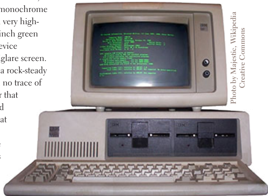
IBM PC 5150 with keyboard and green monochrome monitor (5151), running MS-DOS 5.0
