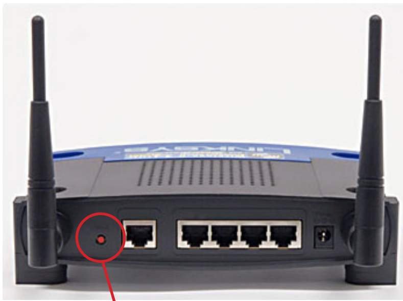
Reset button on the back of a Linksys router
